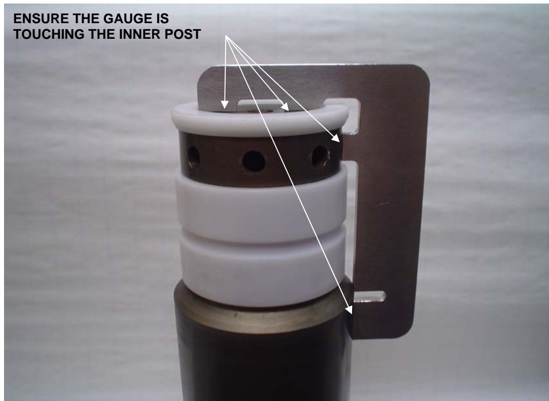
FIGURE 4 – WELD GAUGE PLACEMENT / USE
