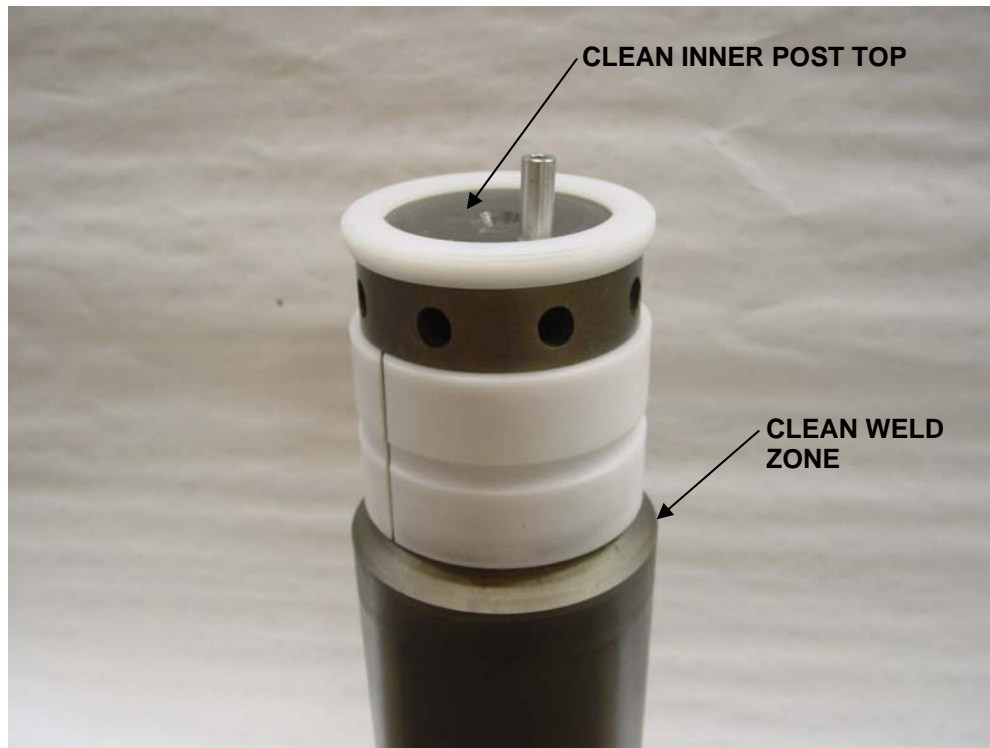
FIGURE 3 – Visually Inspect Weld Zone
