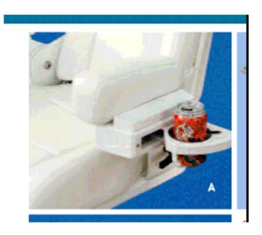
The STIDD Cupholder is attached to either arm by two screws. The arm cushion is removed, the Cupholder attached and then the arm cushion is reattached. Unopened, the Cupholder extends about 2 1/2"; Opened, the Cupholder extends about 7 1/2" off the arm.
