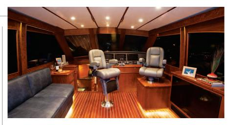
station where the captain can run all the systems. Engine controls include both traditional levers and a joystick with transfer unit and digital readout, along with controls for the ACR spotlight in a lift-open compartment starboard of the wheel. Navigational and fishing electronics are monitored through a small Furuno LCD and an R33 unit in a matching compartment on the port side. Teasers can be adjusted from the station via a
